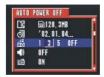
3. Then press the LEFT/RIGHT button ( ) to select OFF / 1 MIN. / 3MIN. or 5MIN. Press the SET button to confirm your selection.
